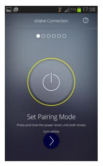
Now with the shower turned off, **press the actual shower Power knob and keep it pressed for 5 seconds**, as illustrated below. Both the Power knob and Flow knob should turn yellow and stay yellow.
